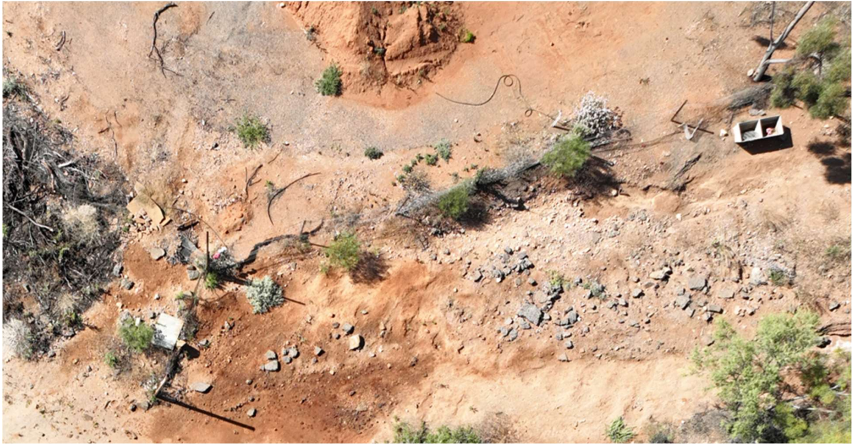
Some Construction waste, mostly Concrete (may fall outside of property)
